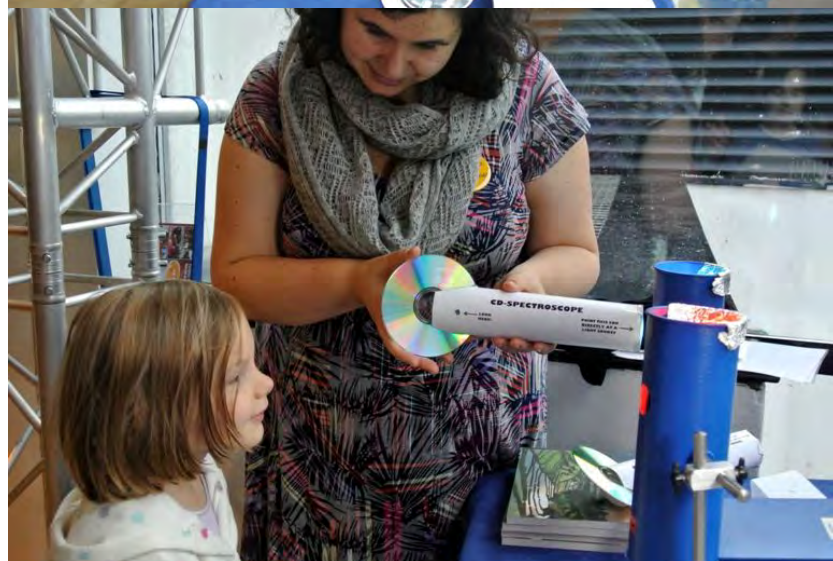
Make your own spectrograph! In this demo visitors could make their own spectrographs using old CDs as gratings to unravel the light. Visitors could then test their spectrographs by aiming them at special gas lamps, and compare the emission line spectra they saw with our printed versions. Images courtesy of T. Fitzpatrick.
